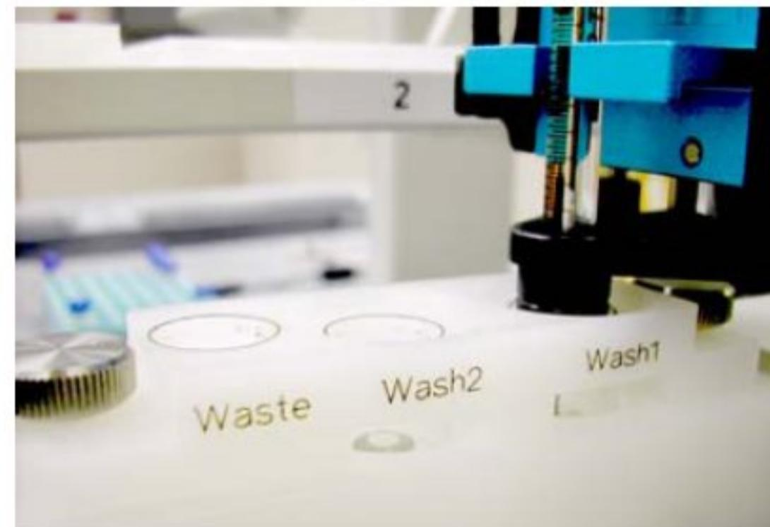
(needle inside and rinsed in a Wash Station different cleaning solvents. This unique design virtually eliminates sample carryover and adsorption problems.
